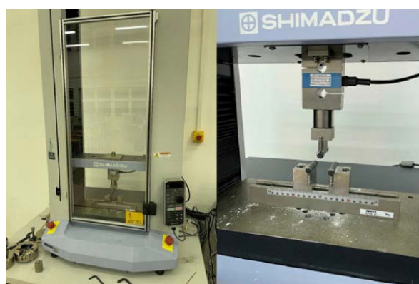
Figure 3. Universal testing machine Shimadzu AGX-V
