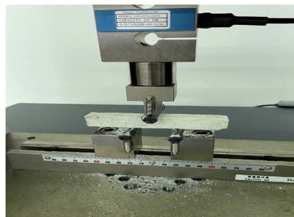
Figure 4. Three-point bending fixture with the specimen placed in position
