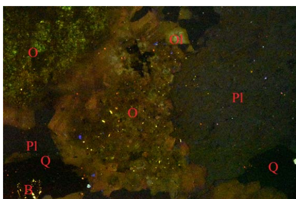
Figure 5. Strong luminescence activity of orthoclase and lack of emission in plagioclase (sample 4; symbols used: O—Orthoclase, Pl—Plagioclase, Ol—Olivine, Q—Quartz, B—Biotite)
