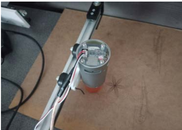
Figure 5. Laser installation (Next to the laser, a test pattern is visible, which was used to determine the initial calibration of the laser and plotter)
