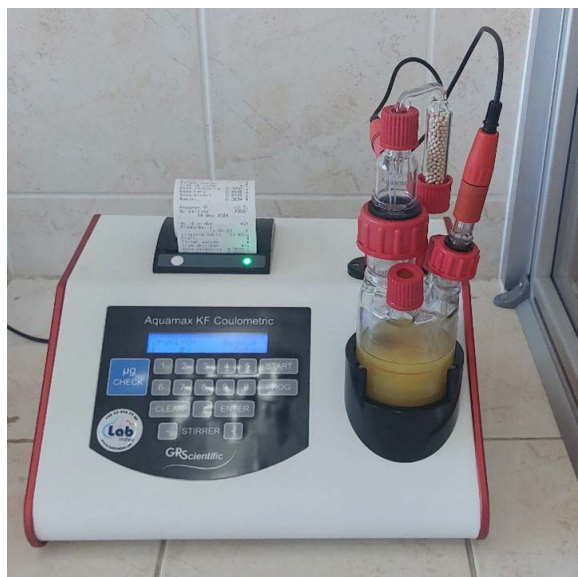
Figure 1. Coulometer for the determination of water content in oil samples by the Karl Fischer method
