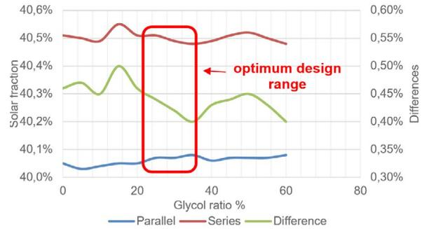
Figure 4. Glycol ratio effect on the solar fraction
