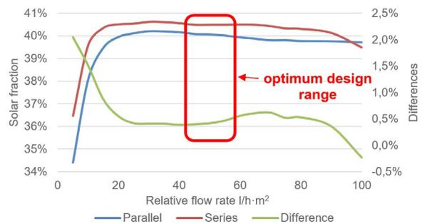
Figure 5. Relative flow rate effect on the solar fraction
