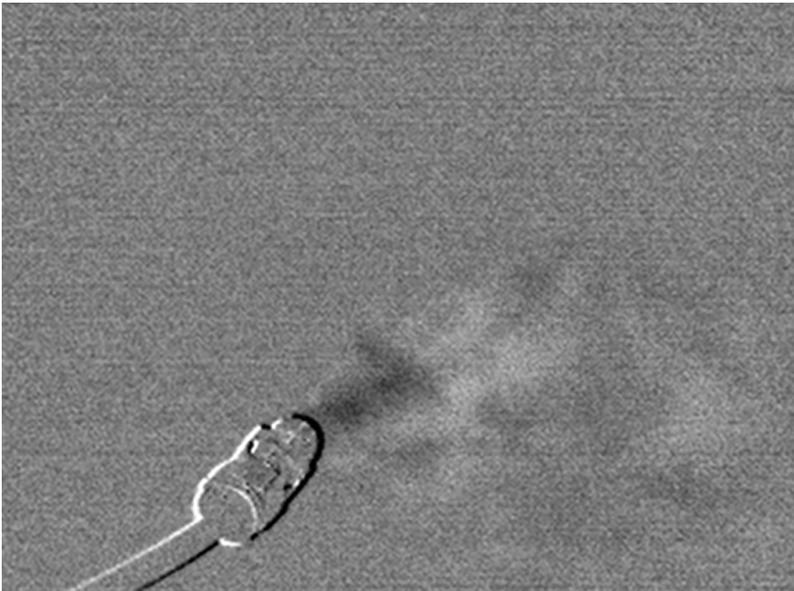
**Figure 9.** Highly sensitive differential mode (HSM) thermogram of **turbulent** emissions of ammonia at 7000 ppm at the ambient temperature of 20°C, against the **background area at 6°C**. FLIR GF306 camera
