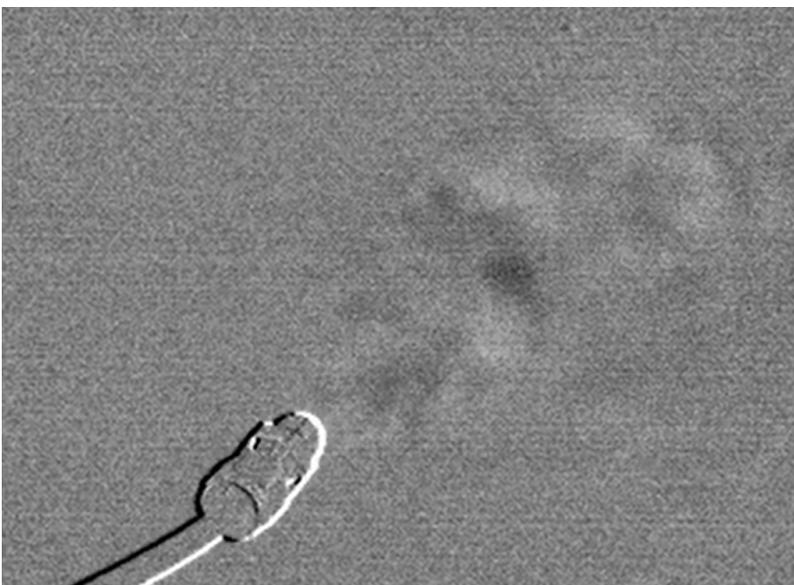
**Figure 10.** Highly sensitive differential mode (HSM) thermogram of **turbulent** emissions of ammonia at 7000 ppm at the ambient temperature of 20°C, against the **background area at 6°C**. FLIR GF306 camera
