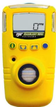
**Figure 3.** GasAlert Extreme Ammonia Meter - detector; [11]
