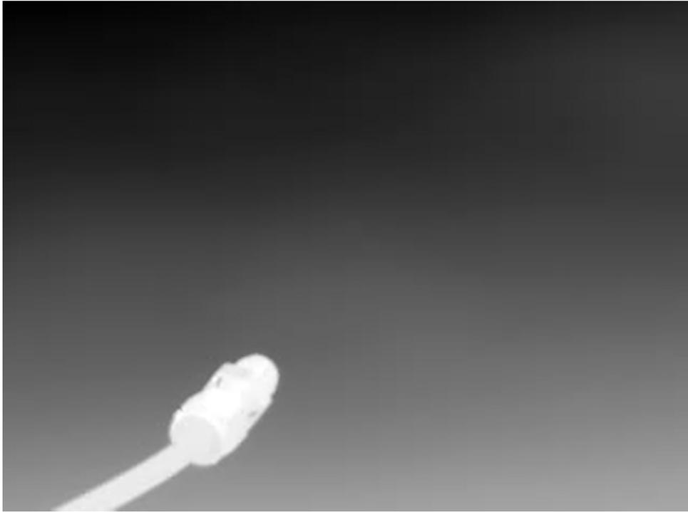
**Figure 6.** Thermogram of laminar emission of ammonia at the concentration of 3000 ppm, at the ambient temperature of 20°C in the background area at 6°C. FLIR GF306 camera
