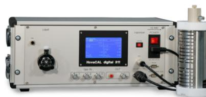
Figure 2. HovaCal – calibration gas generator; [10]
