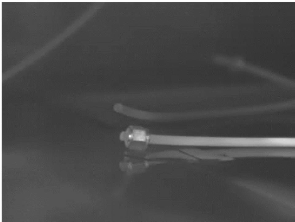
**Figure 4.** Thermogram of laminar emissions of ammonia at the concentration of 300 ppm, at the constant ambient temperature of 20°C. FLIR GF306 camera
