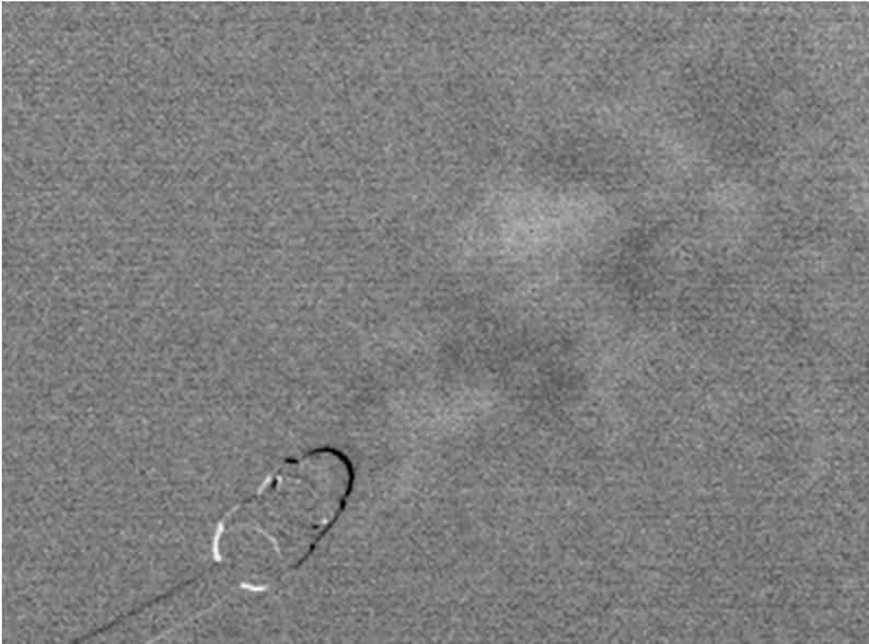
**Figure 8.** Highly sensitive differential mode (HSM) thermogram of **turbulent** emissions of ammonia at 7000 ppm at the ambient temperature of 20°C, against the **background area at 6°C**. FLIR GF306 camera
