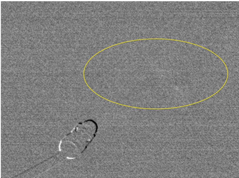
**Figure 7.** Thermogram of laminar emission of ammonia at the concentration of 3000 ppm, at the ambient temperature of 20°C in the background area at 6°C. FLIR GF306 camera
