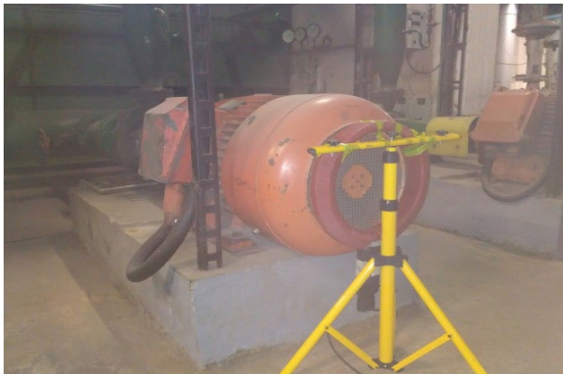
Figure 2. The method of measuring an axial flux at the work place – a coil on a tripod
