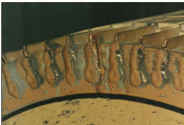
Figure 11. Broken end ring of the 800 kW, 6 kV, 745 rpm induction motor with RFI=2.15
