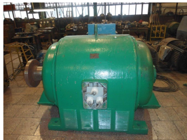
Figure 24. 630 kW, 6 kV motor with built-in coil
