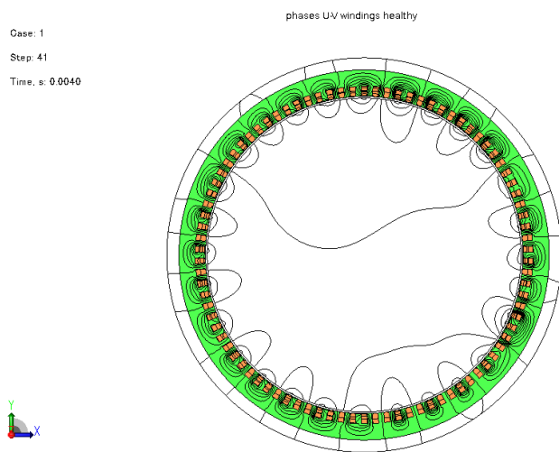
Figure 23. View of the stator cross section of the modeled generator in the JMAG program, flux distribution a) electrical symmetry of the windings – magnetic flux present in the center of the stator
