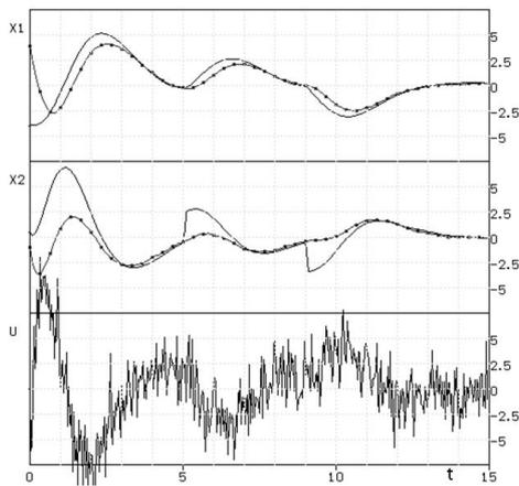
Figure 9. State stabilization with LQR and KF MWO with measurement noise
