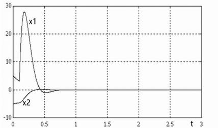
Figure 8. Stabilization of system (32) with LQR and reconstructed state  $x_1(t)$  and  $x_2(t)$  by the use of MWO observer  $T=0.1$
