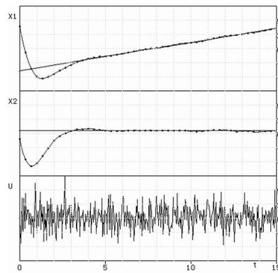
Figure 6. Estimation of the state variables (32) with the measurement noise in control by the use of Kalman Filter
