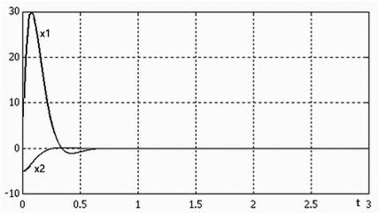
Figure 7. Stabilization of the state in system (32) from nonzero initial conditions with the use of LQR and direct measurement of the state  $x_1(t)$  and  $x_2(t)$  (without the observer)
