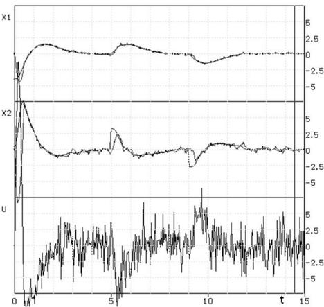
Figure 10. State stabilization with z LQR and MWO with  $T=0.5$ , with measurement noise
