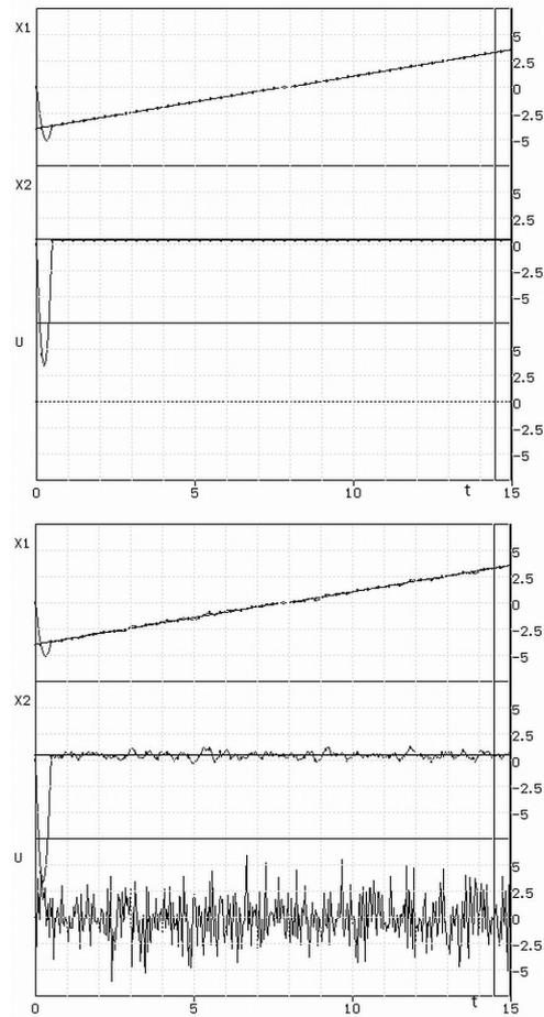
Figure 5. Reconstruction of the state variables  $x_1, x_2$  without measurement noise in  $u(t)=1(t)$  (upper plots) and with measurement noise (lower plots). Left Fig. for MWO  $T=0.5$ , right Fig. for MWO,  $T=1.0$
