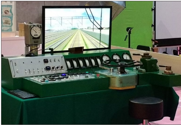
Figure 1. Photo of the ET22 locomotive simulator
