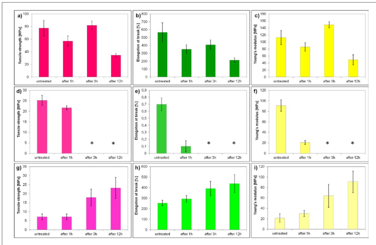
Figure 5. Effect of hydrogen peroxide/UV treatment on mechanical properties of pure PU (a, b, c), of pure PLA (d, e, f) and of PU/PLA (g, h, i). Asterisks indicates the mechanical properties were below limit of detection of used equipment
