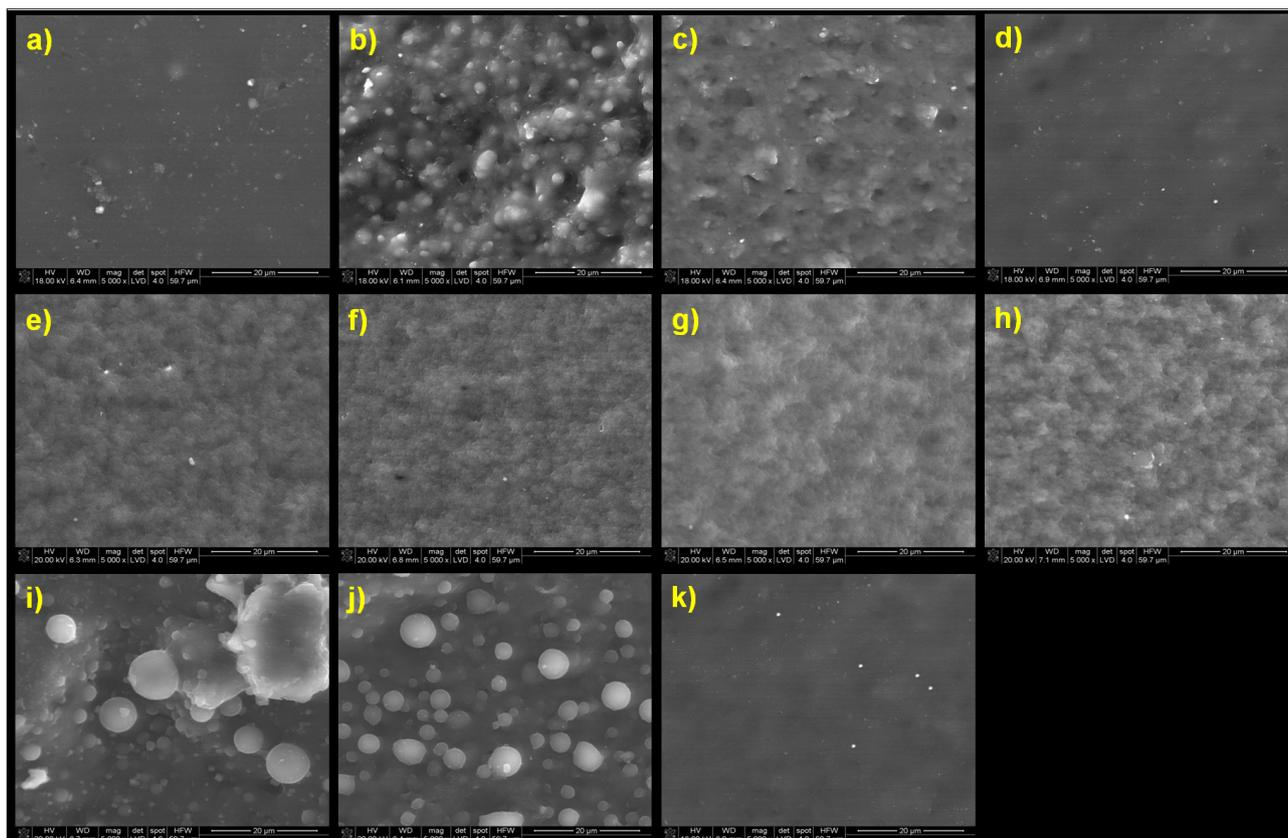
Figure 6. SEM images of pure PU (a) untreated, b) after 1 h, c) after 3 h, d) after 12 h), pure PLA (e) untreated, f) after 1 h, g) after 3 h, h) after 12 h) and of PU/PLA (i) untreated, j) after 1 h, k) after 3 h) hydrogen peroxide/UV treatment
