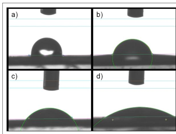
**Figure 2.** Drop shape of pure PU a) untreated, b) treated with hydrogen peroxide for 1h, c) treated with hydrogen peroxide for 3h and d) treated with hydrogen peroxide for 12h
