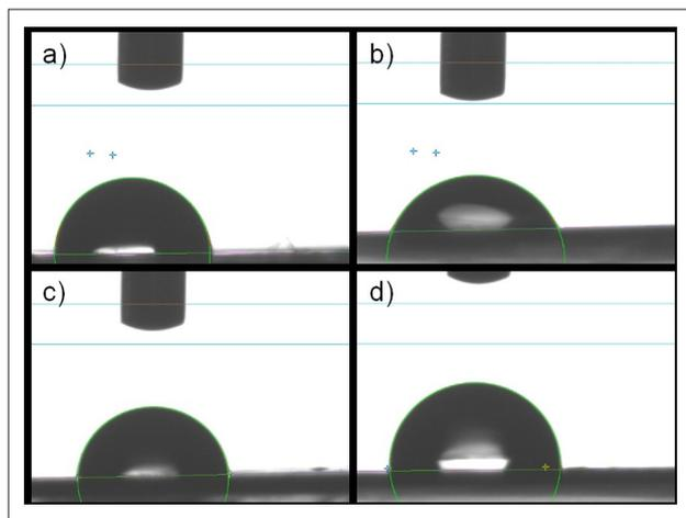
**Figure 3.** Drop shape of pure PLA a) untreated, b) treated with hydrogen peroxide for 1h, c) treated with hydrogen peroxide for 3h and d) treated with hydrogen peroxide for 12h
