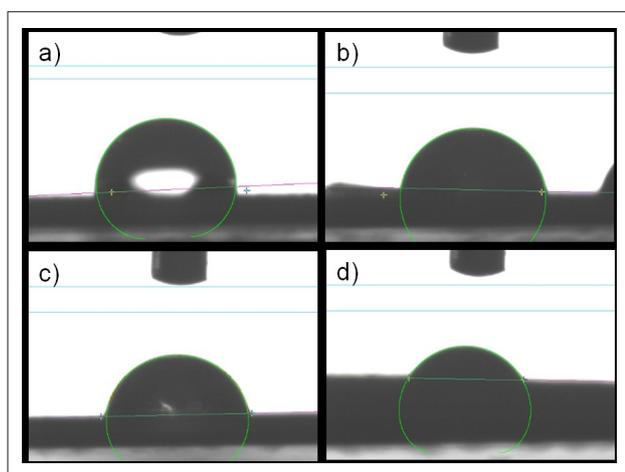
**Figure 4.** Drop shape of pure PU/PLA a) untreated, b) treated with hydrogen peroxide for 1h, c) treated with hydrogen peroxide for 3h and d) treated with hydrogen peroxide for 12h
