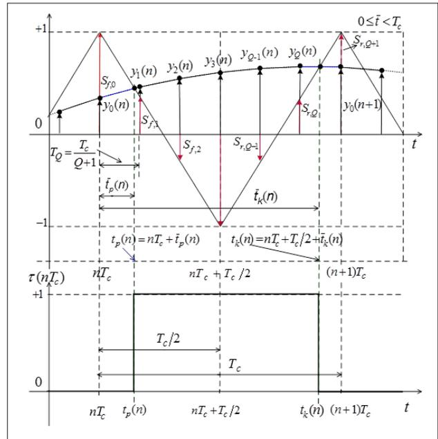
Figure 2. Piecewise linear approximation of the digital audio input for odd  $Q = 5$ .
