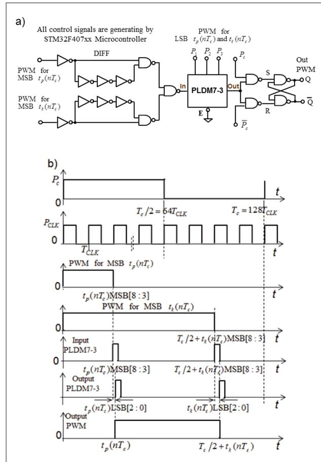
Figure 5. Architecture of the circuit converting 3-LSB (2:0) bits of the data - using a quantizer system based on the 3-bit PTDL. (a) and time domain waveforms of the control and output signals (b)
