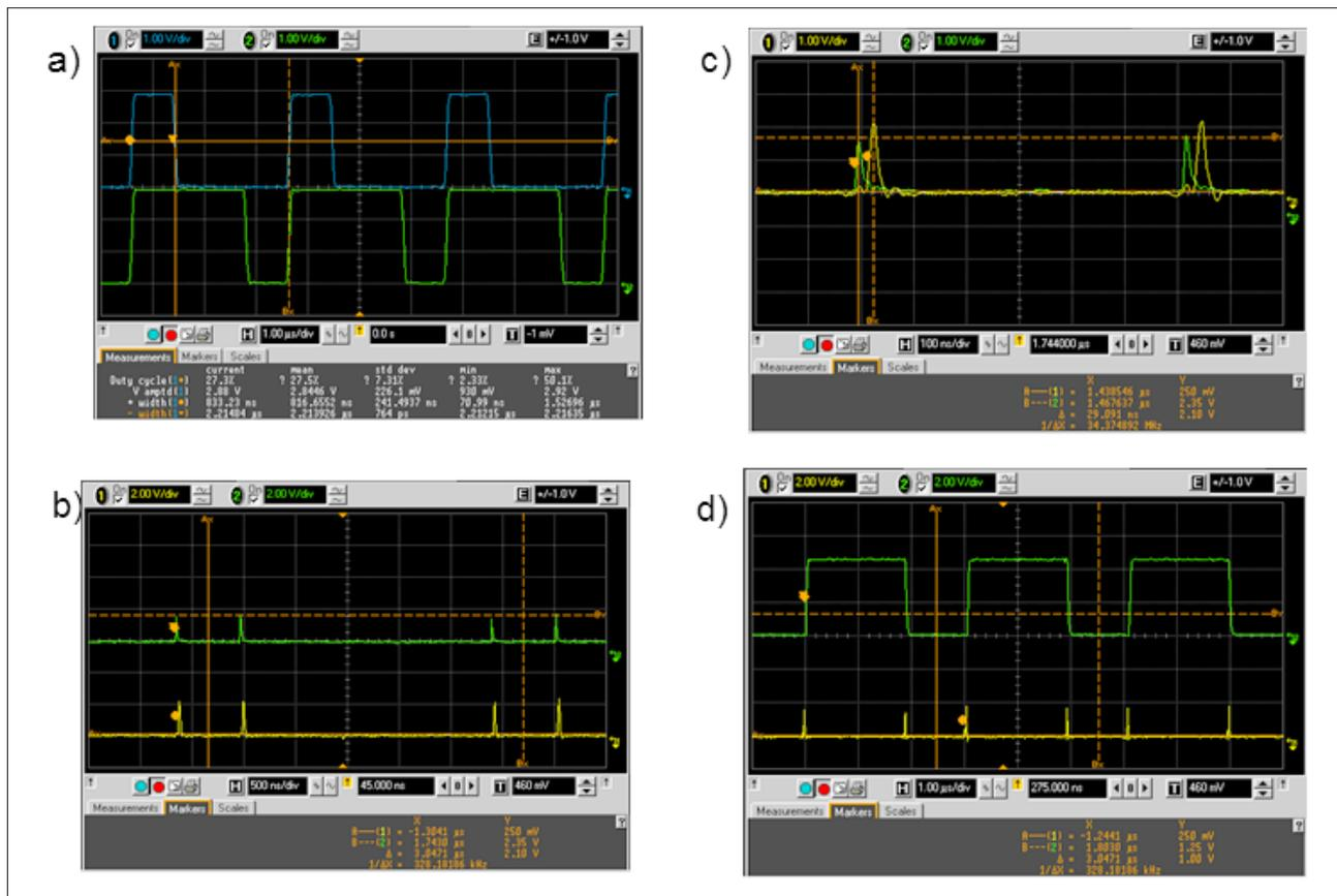
Figure 8. Oscilloscopes of the time domain waveforms of the selected control and output signals, generating by the proposed 9-bit LBDD modulator.
