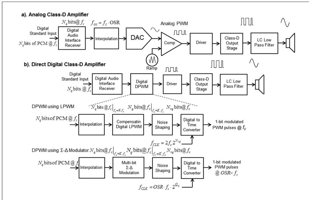
Figure 1. Comparison of analog (a) and direct digital (b) Class-D amplifiers
