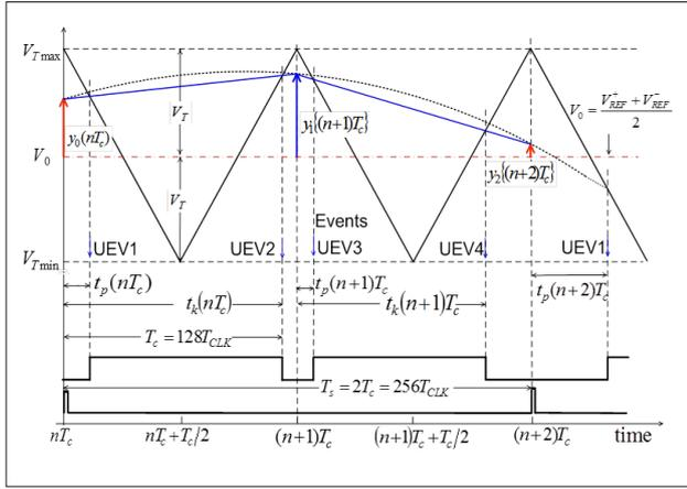
**Figure 6.** Piecewise linear approximation of the digital audio input together with marked locations of update events UEV1–UEV5.
