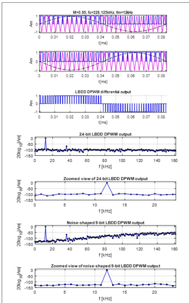
**Figure 7.** Comparison between spectral content of the 24-bit DPWM output and spectral content of the noise shaped 9-bit DPWM output at:  $M = 0.95, f_c = 328,1$  kHz,  $f_m = 12$  kHz for: a)  $Q = 0$ , b)  $Q = 1$ .
