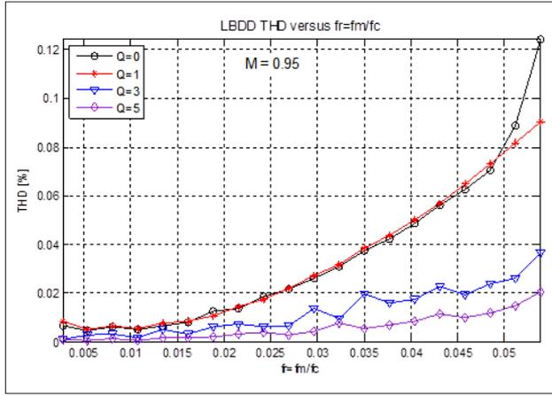
**Figure 3.** THD of the LBDD digital output versus  $f_r = f_m / f_c$  for different  $Q$  values
