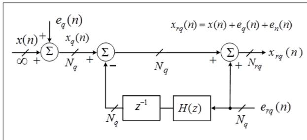
**Figure 4.** Model of noise shaping architecture
