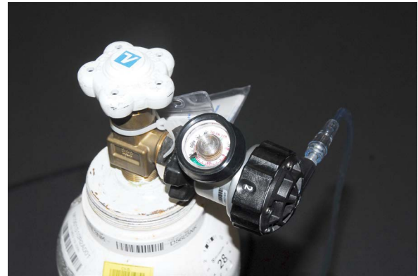
Figure 2. OM-824 Oxygen Conserving Device, the switch (scale 1 to 6) regulates the amount of oxygen applied to every breath (for details see Table 2)
